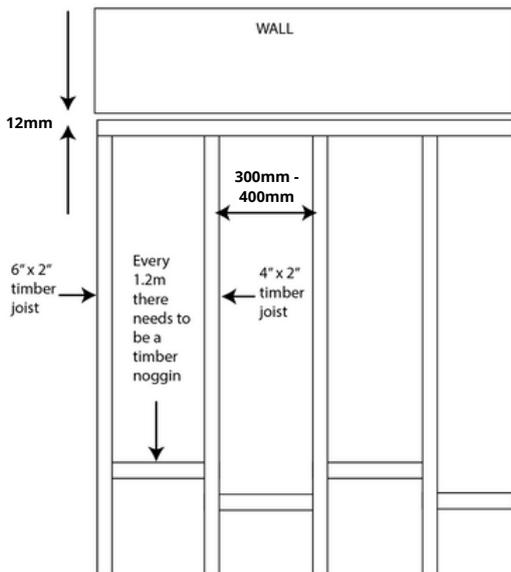
You will need to construct a framework using tanalised timber to support your decking. Leave a 12mm gap between the edge of the framework and any adjoining walls to allow for air flow and heat expansion, or any fixed edge detail (e.g. spindles)
