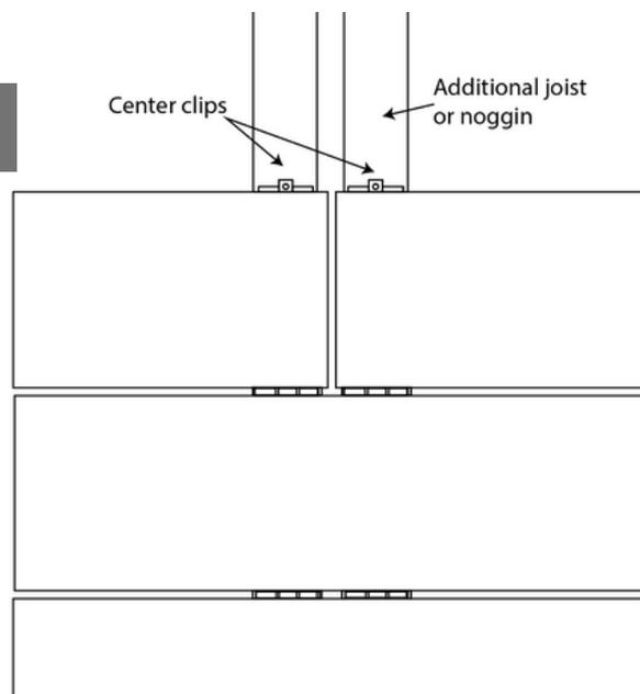
If you need to butt two boards together, ensure that the ends of both boards have their own clip. An additional joist or noggin will be required as support. The clips must be located 15mm in from the end of each board. Allow a 6mm expansion gap between boards (9mm if installing in cold weather).
