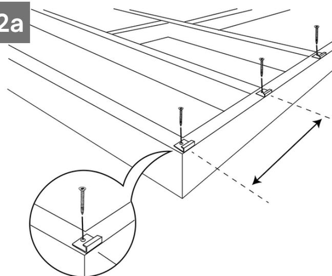
If you are starting with a standard Gronodec board, then locate the starter clips in line with the joists in the position you want to install your first board and firmly secure in place with the screws provided.
