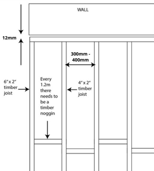
You will need to construct a framework using tanalised timber to support your decking. Leave a 12mm gap between the edge of the framework and any adjoining walls to allow for air flow and heat expansion.
