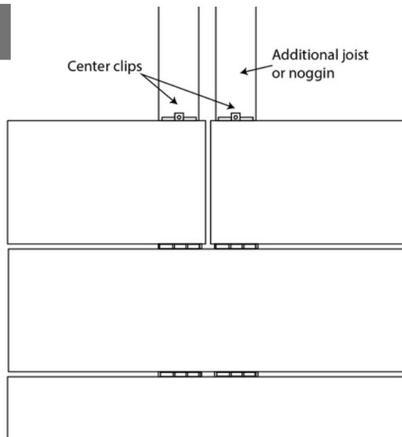
If you need to butt two boards together, ensure that the ends of both boards have their own clip. An additional joist or noggin will be required as support. The clips must be located 12mm in from the end of each board. Allow a 6mm expansion gap between boards (9mm if installing in cold weather).
