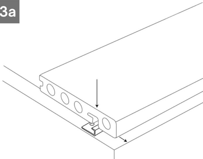
Locate the groove of the Gronodec edging board above the starter clip and lower into position, gently push the board forward into the locked position.
