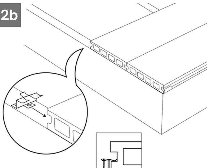
Next push all centre clips firmly into position along the groove of your Gronodec board in line with joists and secure tightly with screws. Locate the next board in position and push it firmly into the centre clips until locked securely in place. Repeat step 2b until all boards have been secured.
